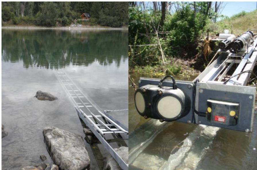
Figure 1. Rail deployment system for Acoustic Velocity Meters (photo courtesy of Molly Wood).
